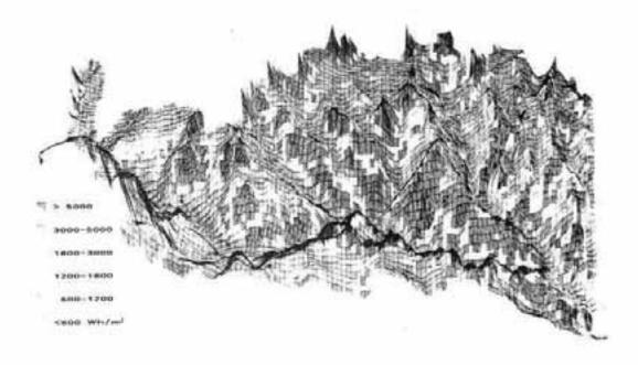
Fig. 2 - Solar radiation map of the middle and high Orco Valley on January 15 (isometric view).
